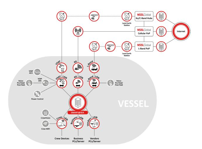
SMART@SEA is designed to give maritime customers complete control regardless of the satellite or terrestrial communications system on-board.
